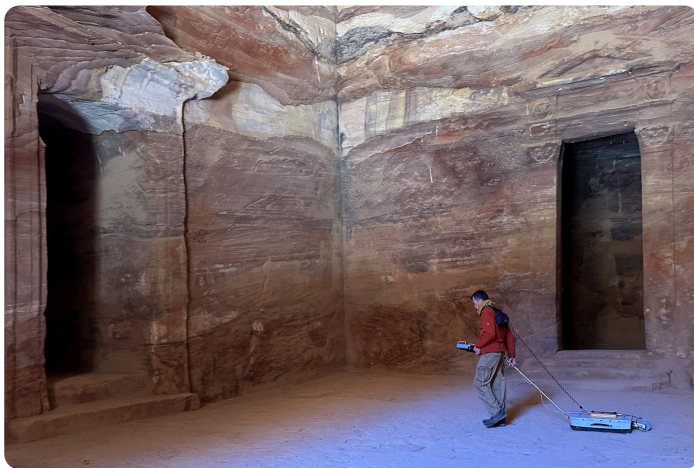
Fig. 5: Ground-penetrating radar scanning within the main chamber of the Treasury. (Photo by M. Vincent.)
